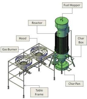
burned rice husks; and (4) a char pan which holds the char prior to disposal. The gas produced from the reactor is burned in the drum-type gas burners to produce a luminous blue-to-pink
