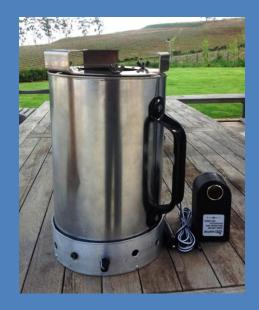
The Khaya Cooker is a Biomass Gasifier Stove that uses a small fan to control the burn of the pellets and produce a smokeless flame.
