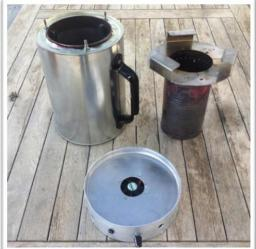
to forced air into the fire chamber. The air is directed through primary holes in the bottom of the chamber to assist in the release of the wood gasses which are burned off near the secondary holes. See next section for explanation of the stove operation.
