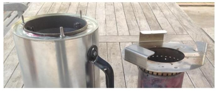
Once the fire chamber has been positioned and attached, the stove top is lowered into the stove body onto the positioning screws. The 3 wing nuts are then tightened ensuring that the secondary air flow from the fan rises on the outside of the chamber, heats up and then is fed through comb into the top of the stove where it mixes with the released gasses.
