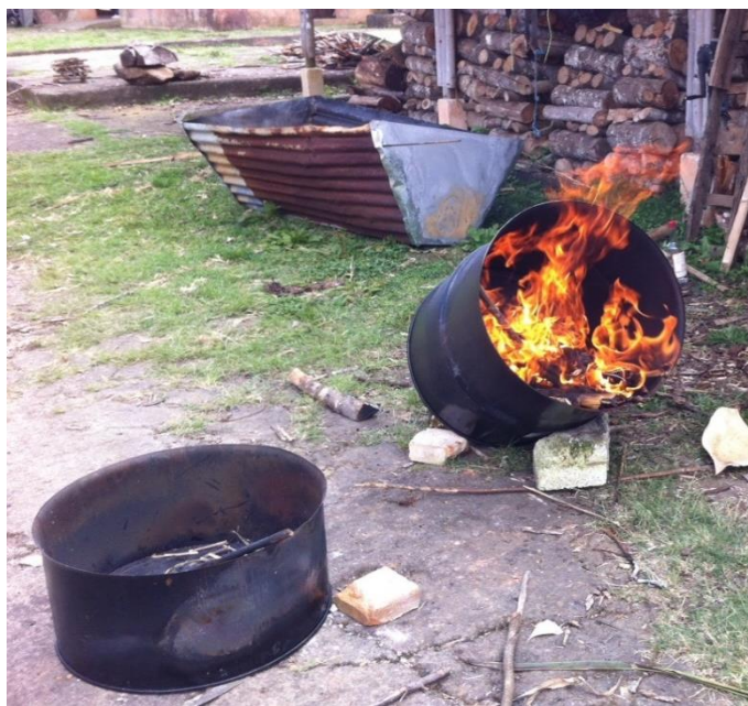
Figure 4: Two FC tubs from one 200 L barrel and a FC trough with 600 L capacity in the background.
