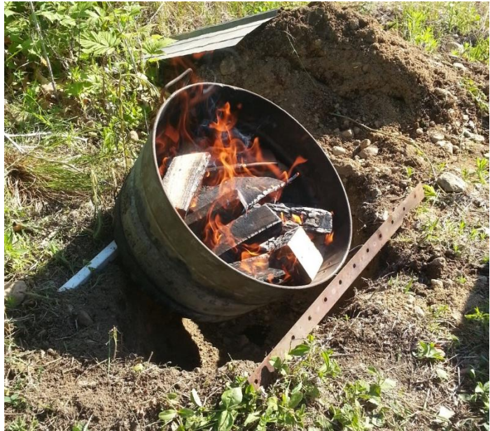
Figure 1: A Flame Cap (FC) Tub Char Maker, by Bruce Southerland, NH. (approx. 2015)
