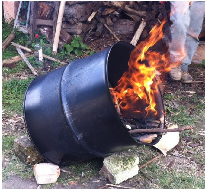
Figure 3: This FC tub is 2/3 rd of a 200 L barrel. For initial use, the barrel was inclined and supported with stones and blocks placed underneath the ribs.
