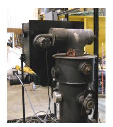
The combustible gases and flames exit from the top of the gasifier, assisted by the induction fan (shown), and can be directed in any direction, including downward on the outside of the Dragon unit. Literally, "the Dragon puts fire into your application when and where you want it."
