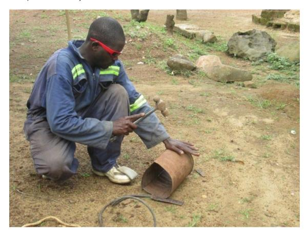
We remade the cylinder by joining two pieces (by welding) of metal pieces, each made into a half circle. The cylinders turned out to be much rounder this time. We did not use any nail or screw in the process. He then measured the holes and cut it again using his machine.
