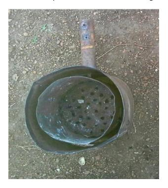
After finishing this part, we make the concentrator lid. This is done by measuring the top part and the side part separately and weld them together. We also made the riser separately. We welded three rebars onto the riser as pot stand. However, we felt that the riser is still very unstable to support the pot, so we decide to weld the riser onto the concentrator lid.
