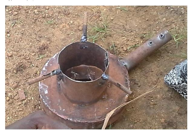
So we are ready to test it. We used wood pieces cut to similar length and filled the gap with dried leaves.
