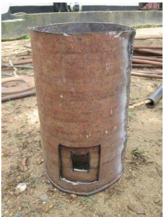
After making both cylinders, he measured and cut a round metal piece to go under the inner cylinder. I asked him to cut the metal piece bigger so that it can actually wrap the bottom part nicely. I also requested him to join both cylinders together. He did this by welding a few long round metal pieces
