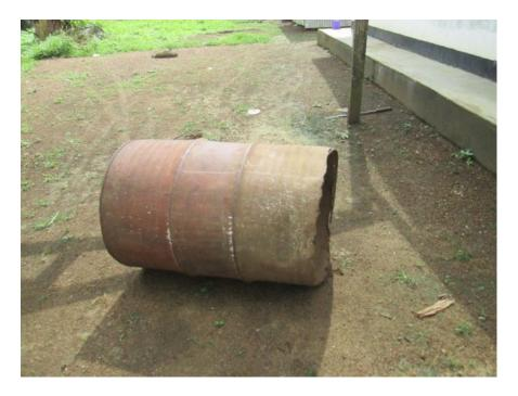
We start by making an outer cylinder. Our welder measured the required length (with several cm extra) of metal to be folded into a cylinder of 18.5cm diameter using a metal ruler. He marked the metal with another metal piece. Then he cut the drum using machine (see picture below).
