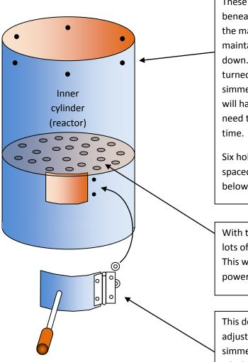
TLUD stoves are difficult to turn down to low power for simmering. The flame cools and goes out at low power levels. These holes allow small pilot flames beneath the main flame which support the main flame, keeping it hot and maintaining flame presence during turndown. This allows the stove to be turned down to low power for simmering. Less fuel is used and so you will have a longer burn time. You will need this to get the 2 hours of cooking time.
