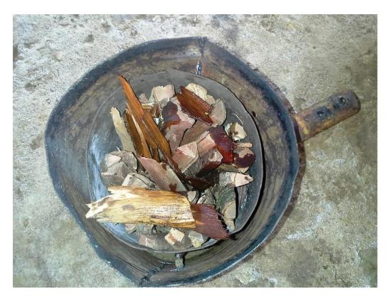
This is how we pack the wood prior to third stove test. From this picture one can see that although we tried to pack the wood vertically, the upper part is still quite loose (having much cavity).
