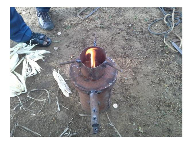
So after some discussion, we decided to make the inner hole of the concentrator lid bigger (as big as the riser diameter), and also cut some holes into the riser in order to have some air space under the pot. See pictures below
