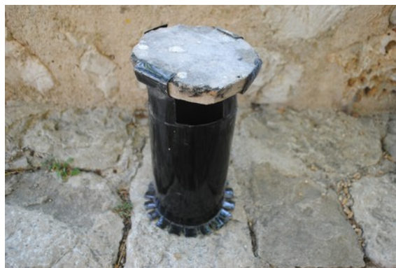
Figure 4. TLUD Riser and diffuser. Diameter: 12 cm. Total length: 30cm. Diffuser: granite piece 2cm thick and 15cm diameter
