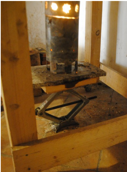
Figure 7. Holding the stove with the jack. Objects below the jack (like the black box) can be added depending on the total height of the stove
