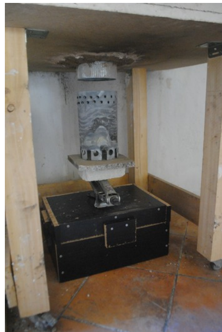
Figure 7. Holding the stove with the jack. Objects below the jack (like the black box) can be added depending on the total height of the stove
