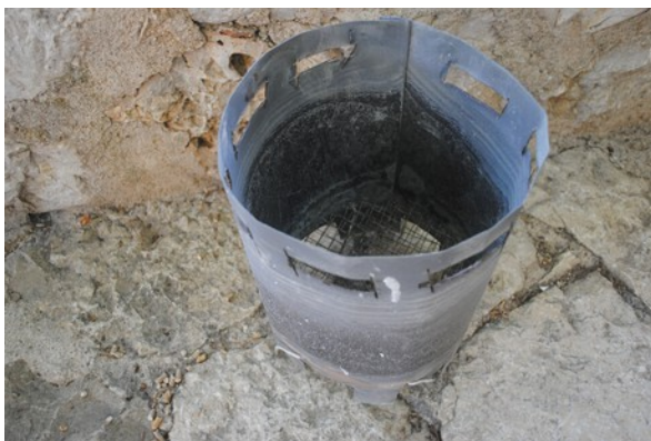
Figure 2. TLUD Reactor. Diameter: 20cm. Total length: 30cm. Fuel Height: 20cm. Primary air entrance is at the bottom and also at 12cm from the bottom through a set of 11 rectangular holes (2,5*0,5cm). Secondary air entrance are 7 rectangular gaps (5*1,5cm)
