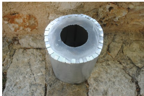
Figure 3. TLUD Outskirt. Diameter: 22cm. Diameter central hole: 12,5cm. Total length: 25cm
