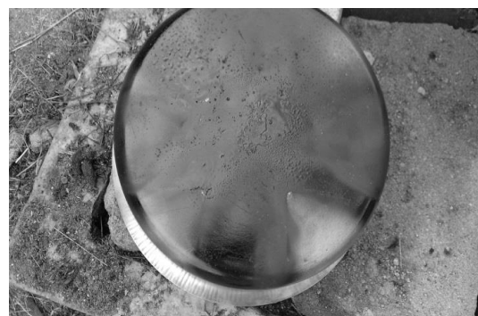
Figure 6. Typical soot with tar on pot bottom after cooking on natural draft TLUD stove with pellets.
