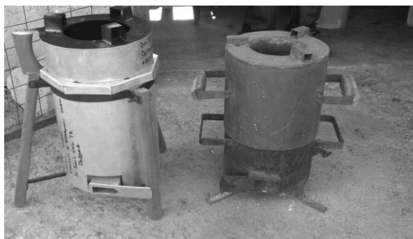
Figure 2. Troika (left) and Jiko Bomba TLUD stoves. Primary air vent can be seen at bottom of both.
