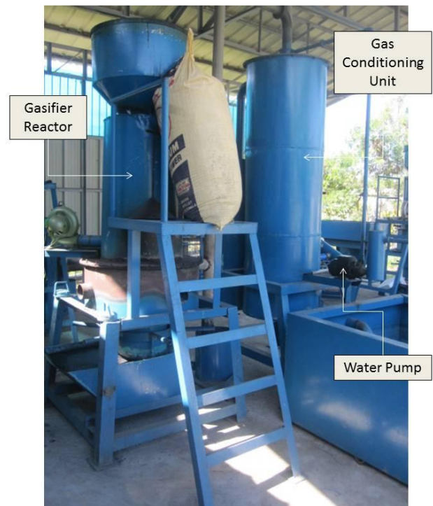
Figure 1. Rice Husk Gasifier with Gas Conditioning Unit Attached.
