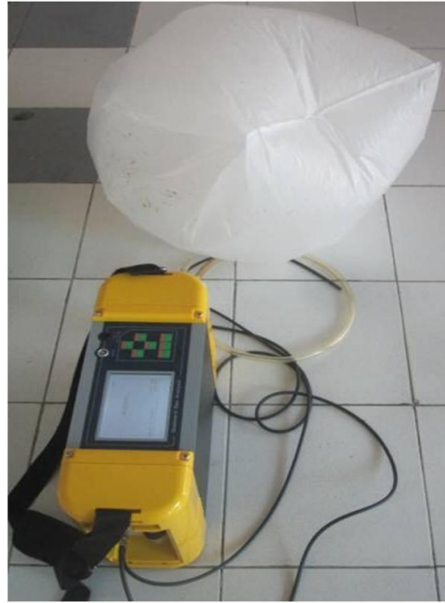
Figure 2. Sample of Gas Taken from the Gasifier and Gas Conditioning Unit and the Gas Analyser Used in the Study.
