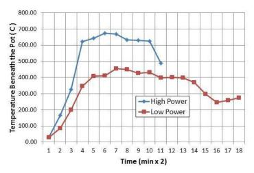
Figure 3. Temperature Profile Beneath the Pot.
