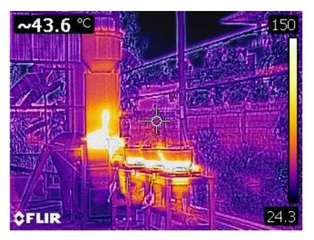
Figure 4. Thermal Image of the Stove During Operation.
