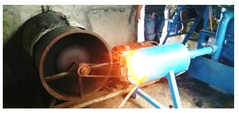
Figure 2. The Gas Burner of the Gasifier During Actual Drying Operation.
