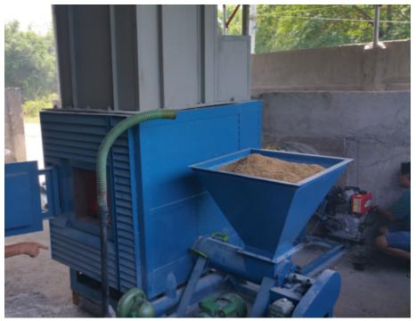
Figure 1. The Char Producing Biomass Furnace.
