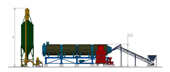
Figure 6. Schematic Drawing of the Torrefying Machine.
