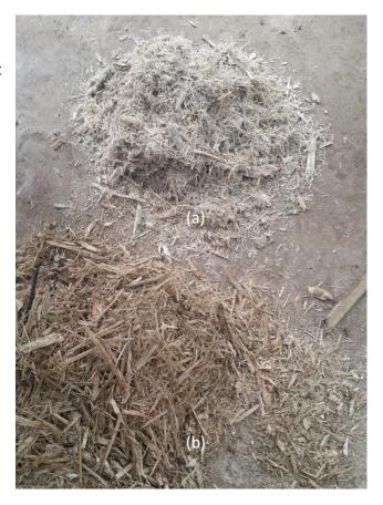
Figure 7. Samples of (a) Raw and (b) Torrefied Sugar Cane Bagasse.
