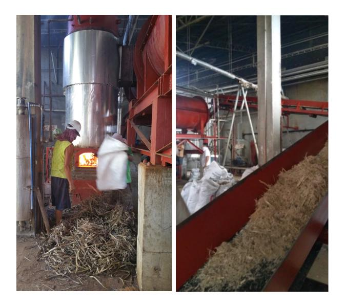
Figure 4. The Biomass Furnace.
