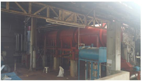
The indirect-fired rotary torrefyer, shown in Figures 1, 2, and 3, was designed to produce torrefied fuel from sugarcane bagasse. It consists of the following major components
