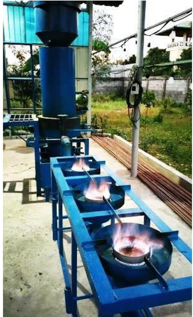
Figure 1. Pictorial View of the CNC Three-Burner RHGS for Small Resto and Food Catering Services.
