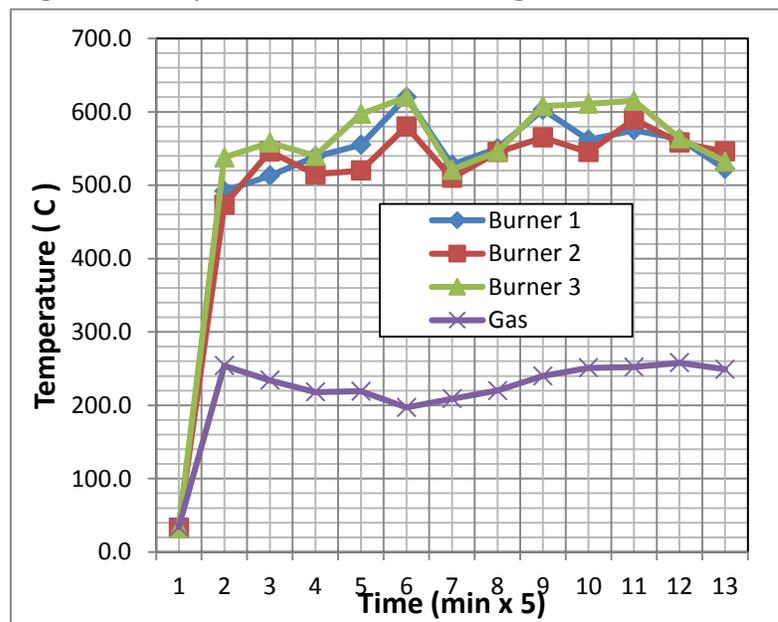
Figure 3. Temperature Profile of the Gas Leaving the Reactor and the Flame Beneath the Pots.
