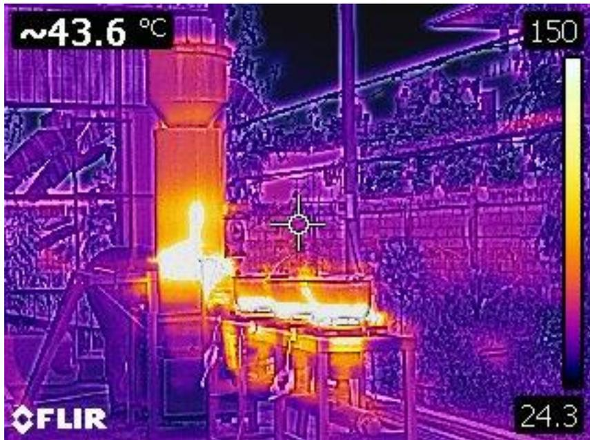
Figure 4. Thermal Image of the Stove During Operation.
