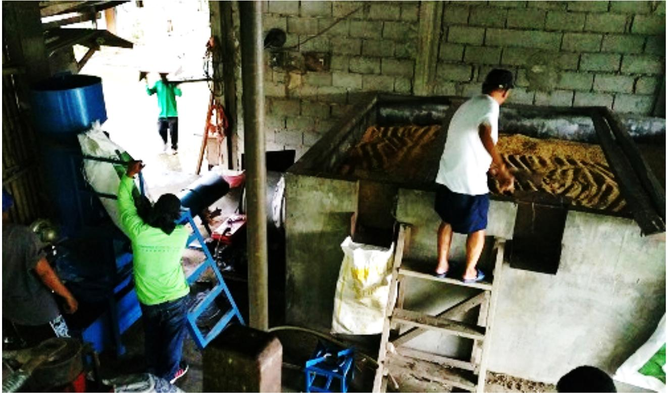
Figure 3. The Gasifier and the Dryer During the Training of Operator and Actual Field Testing.
