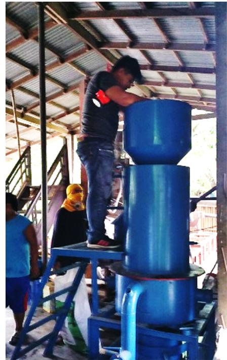
Figure 1. The Model-40D Rice Husk Gasifier Combustor.
