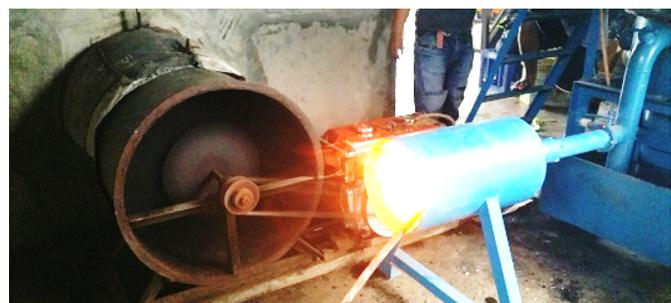
Figure 2. The Gas Burner of the Gasifier During Actual Drying Operation.
