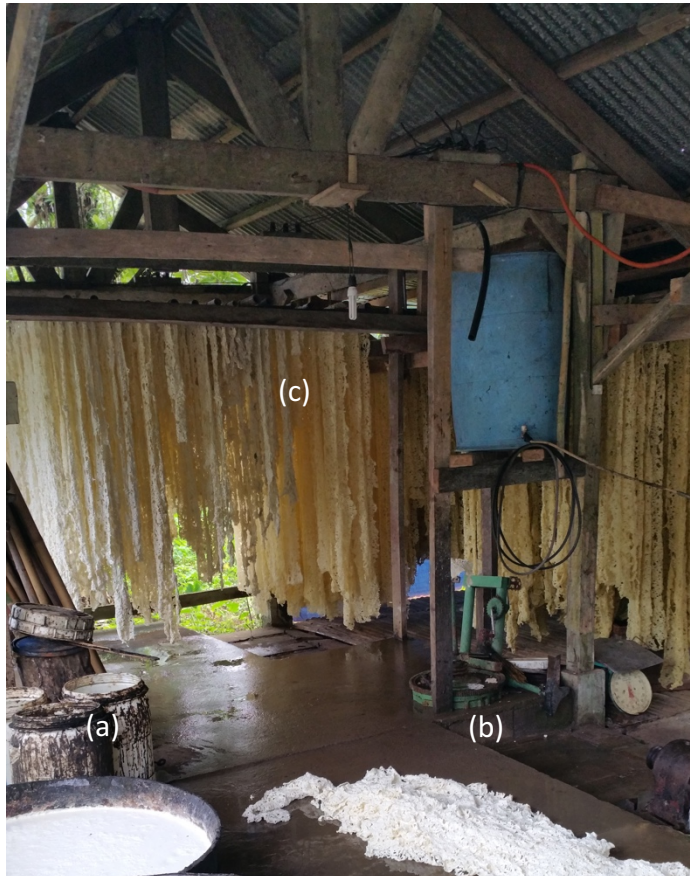
Figure 1. The (a) Fresh Rubber Latex, (b) Newly Pressed Rubber Blanket, and (c) Rubber Blanket Being Dried
