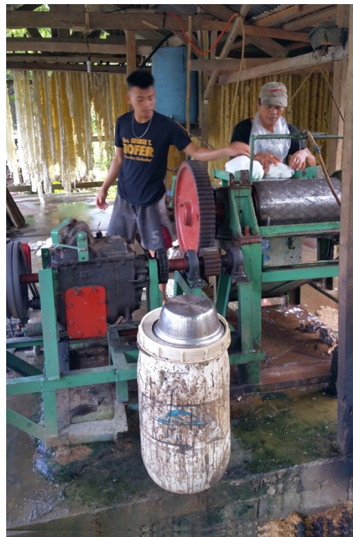
Figure 2. The Diesel Engine Operated Creeping Mill to Produce Rubber Blanket.
