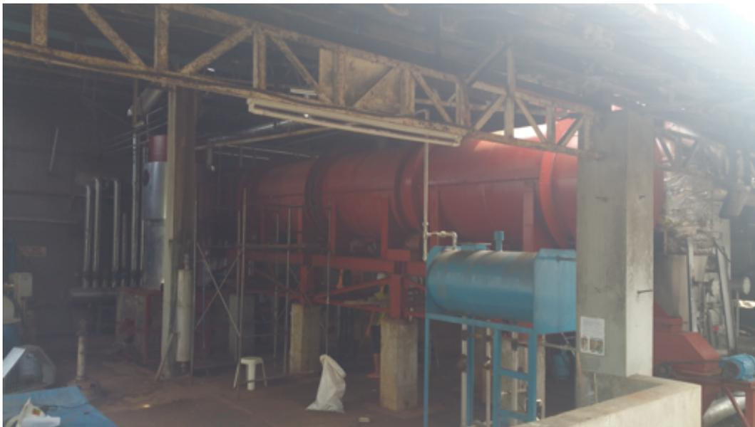
Figure 1 The Sugar-Cane Bagasse Torrefyer (SCRT)
