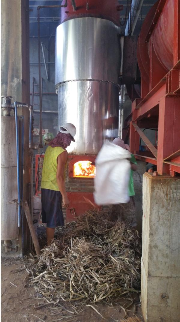
Figure 4. The Biomass Furnace.
