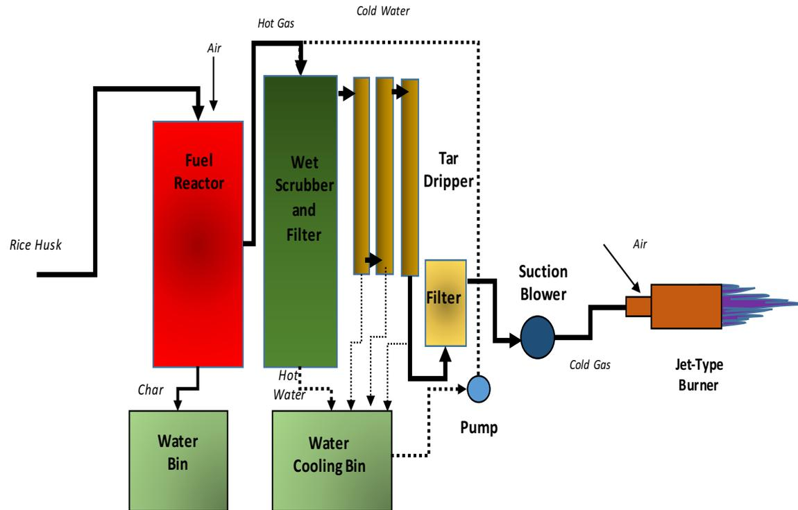
Figure 4. Schematic of the Process of Operation of the Gasifier.
