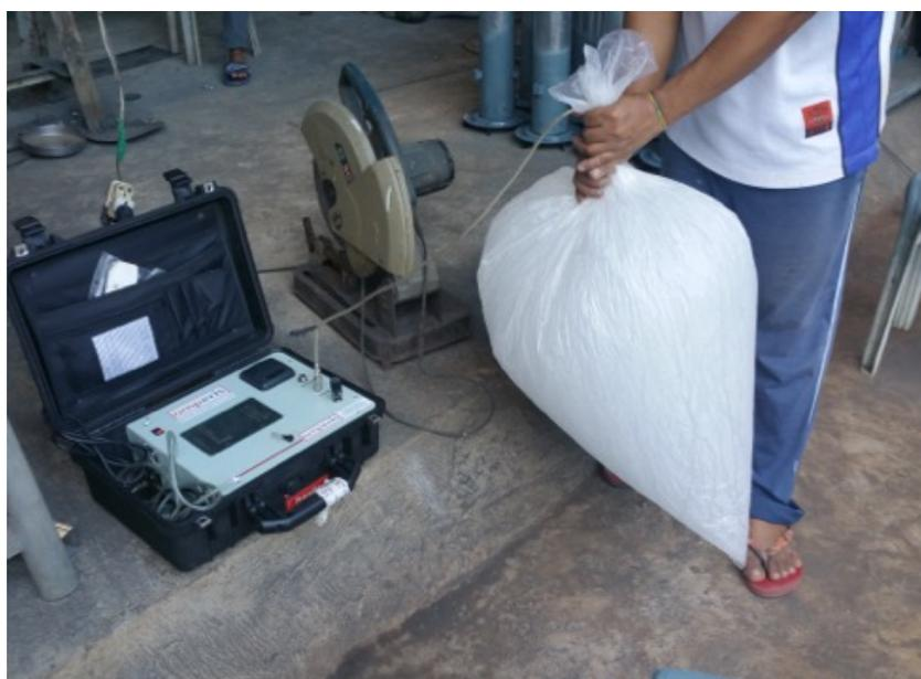
Figure 6. Gas Composition Measurement Using the Amperis Transdox Gas Analyzer.
