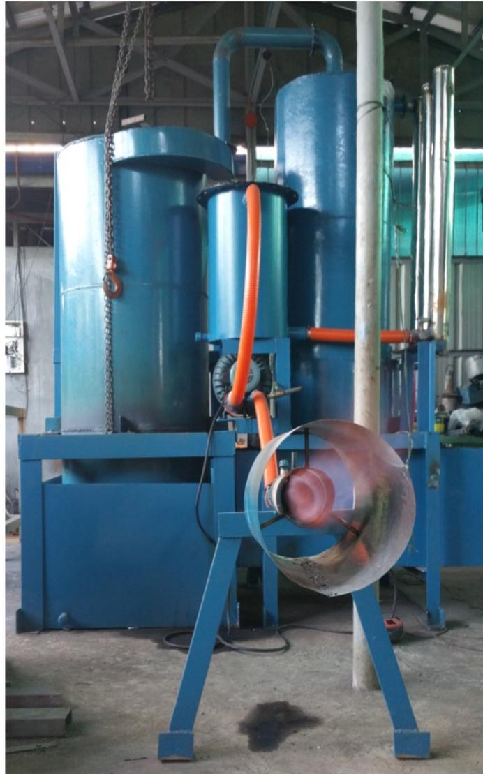
Figure 1. The Induced-Draft Rice Husk Gasifier with Wet-Scrubbing Unit and Jet-Type Burner during Operation.
